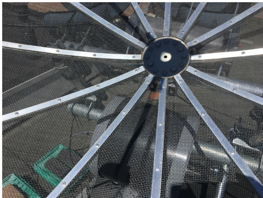
Fig. 6. Shadow of the feed on the dish while tracking the sun. Using this, both the tracking software and the alignment of your system can be checked.
