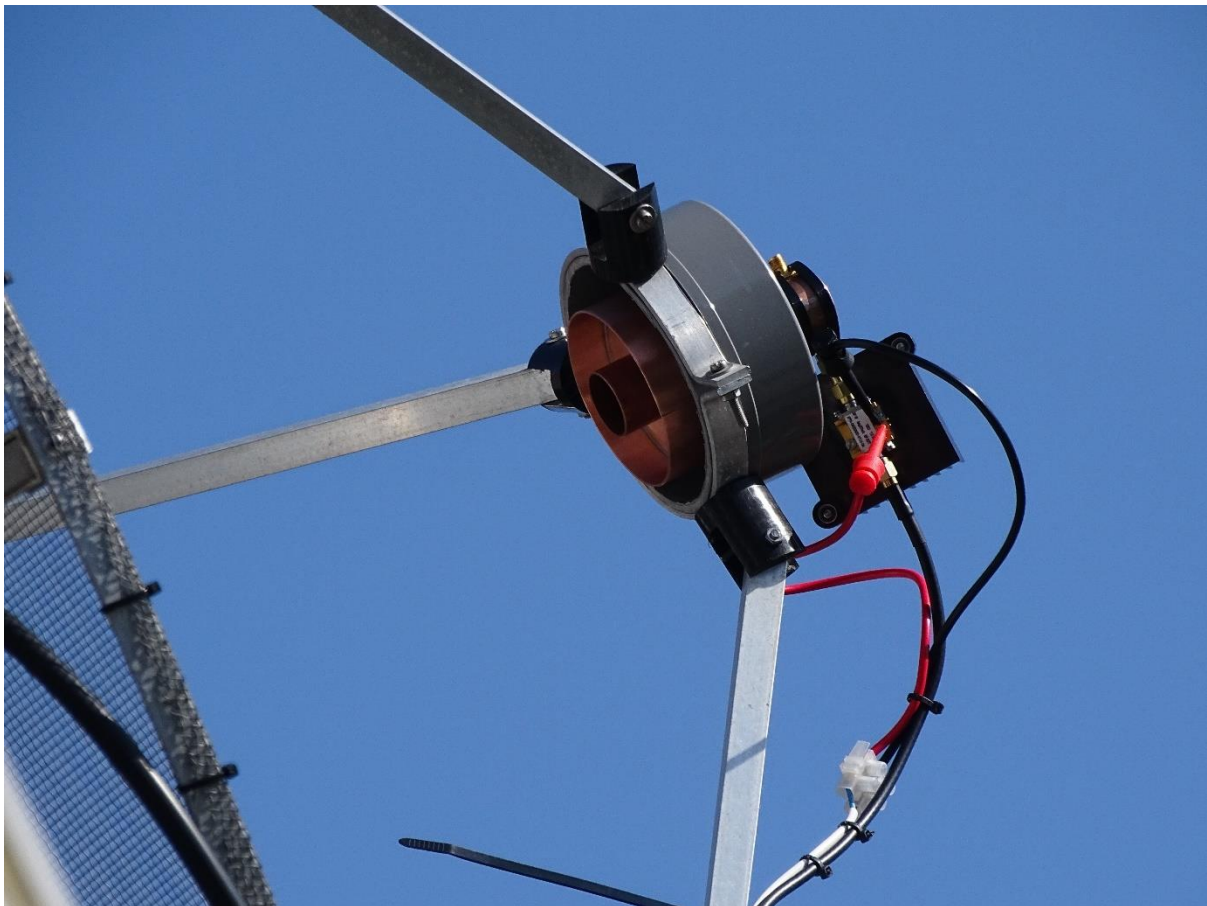
Fig. 3. Feed and LNA as mounted at the dish.
