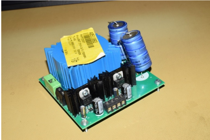
Fig 6 The built-up nutrition. The capacitors are still of the axial type.
