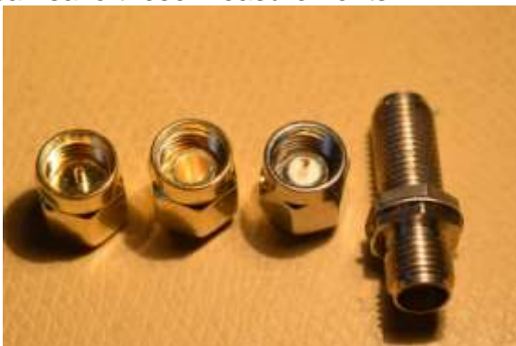
Fig 5 SOLT . From left to right: Short, Open, Load and Through
