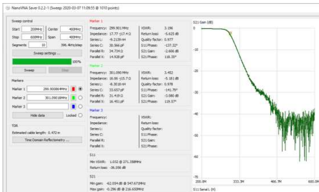
Fig 6 A measurement of a 300 MHz lowpass filter from Mini-Circuits: BLP-300 +
