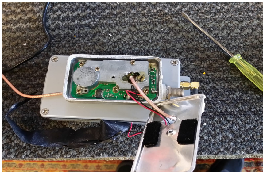
FIG. 1. Converted TV LNB; the bottom box contains a PLL that generates 6300 MHz; see fig. 2.
