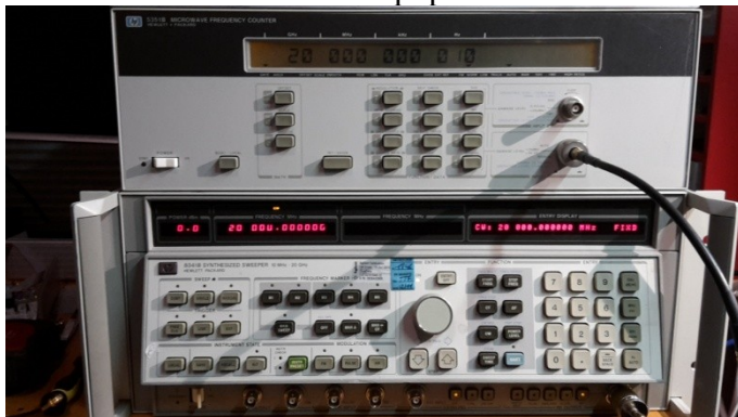
Fig 1 HP8341B Synthesized Sweeper up to 20GHz (including attenuator to -110dB), with above that a HP5351B Microwave Frequency Counter up to 26.5GHz (with OCXO)
