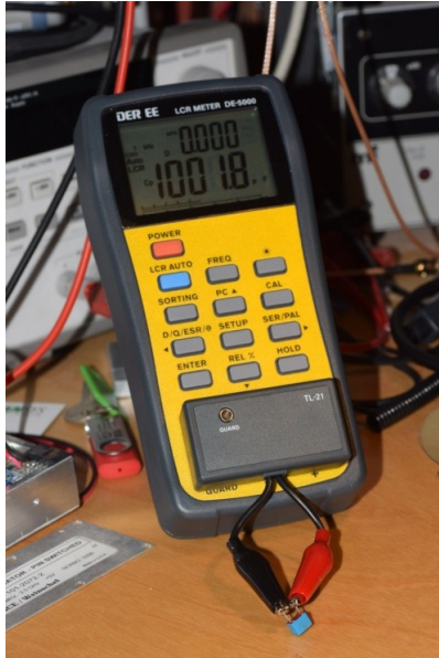
Fig 4 Meter in action with a 1000 pF "precision" capacitor
