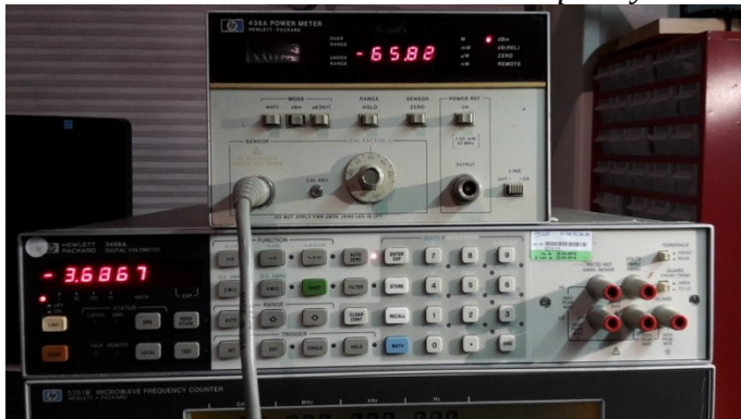
Fig 2 HP436A Power Meter with HP8484A power sensor and above that a HP3556A Digital Voltmeter, 6.5 digits
