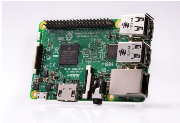
FIG 10 The Raspberry Pi 3. On the right you see 4 USB and the network connections . At the bottom of the print is a micro sd card reader.
