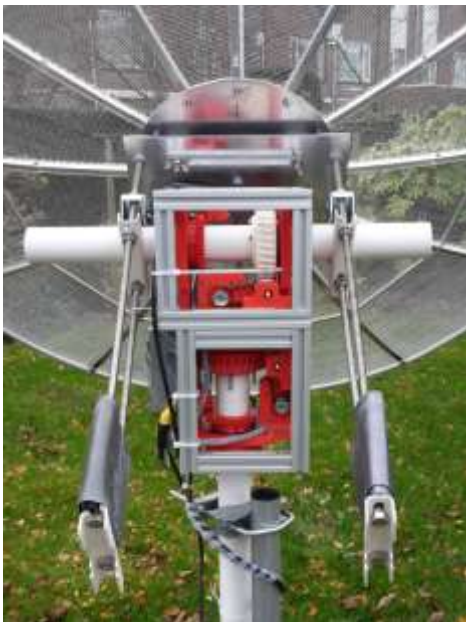
Job self -assembly rotor , with 3D-printed parts and aluminum profiles.
