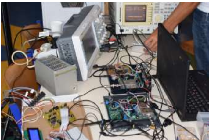
With a QPSK signal generator receivers of Job de Haas and Peter Smits compared
