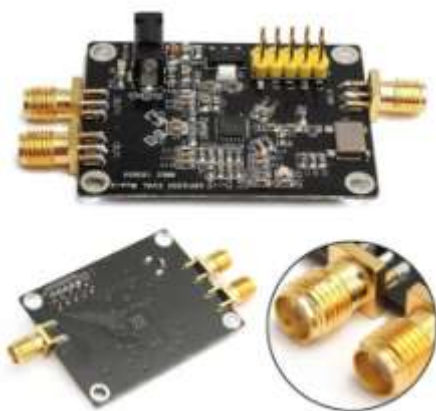
Fig 3 the left, the two outputs, to the right the port for an (optional) clock. If you look closely you see that the SMA connector and not to the bottom soldered.
