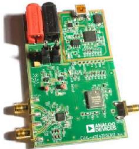
Figure 2 The evaluation board of Analog Devices. The ADF4351 is located at the bottom left. Top right is the Cypress CY7C68013A controller and USB interface.
