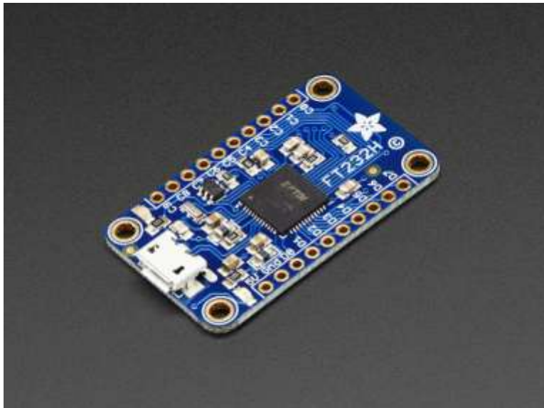
Figure 2 FT232H module of Adafruit. The chip has an on-board regulator 3V3. Unfortunately, this is not available on the pins.
