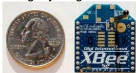
Fig.1 – XBee with wire antenna met 1mW transmission power
