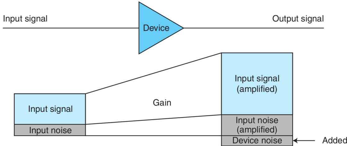
$$\text{Input SNR} = \frac{P(\text{input signal})}{P(\text{input noise})} > \text{Output SNR} = \frac{P(\text{input signal})}{P(\text{total output noise})}$$
