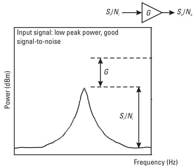
Figure 4.5 Signal-to-noise degradation of a signal passing through a semiconductor device.
