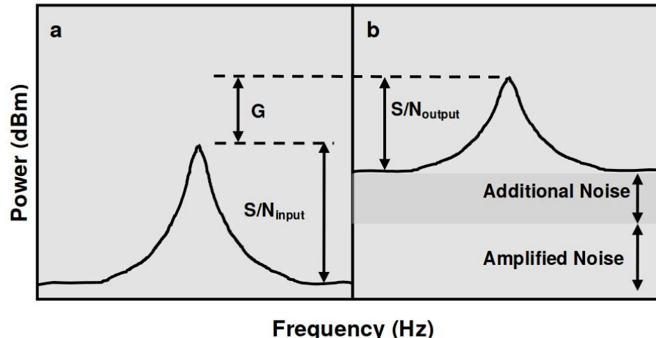
**Figure 1** Signal-to-noise degradation of a signal passing through a semiconductor device. The input signal (a) has low peak power and good signal-to-noise properties. The output signal (b) has a higher peak amplitude, but also an increased noise floor, giving overall poor signal-to-noise performance.
