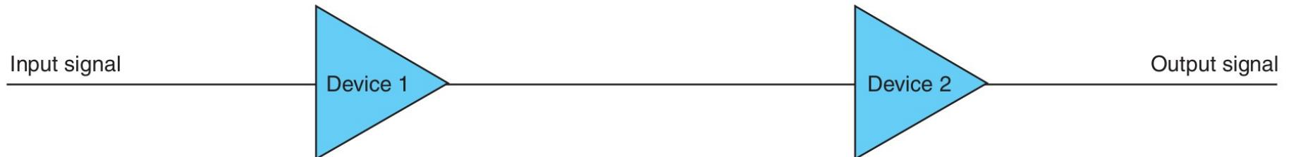
$$F = F_1 + \frac{F_2 - 1}{G_1} + \frac{F_3 - 1}{G_1 \times G_2} + \frac{F_4 - 1}{G_1 \times G_2 \times G_3} + \dots$$
