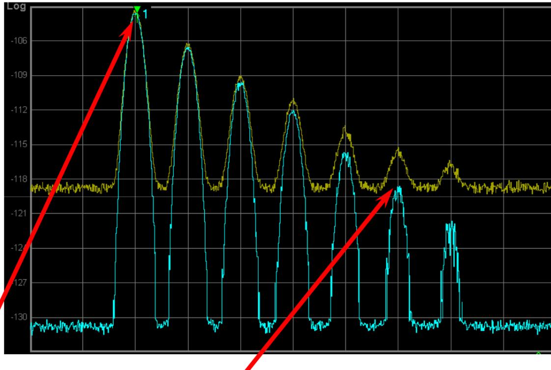
“No” error for best S/N, 3 dB for signal at analyzer DANL
