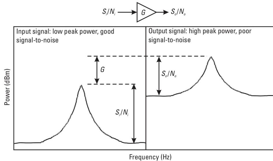
Figure 4.5 Signal-to-noise degradation of a signal passing through a semiconductor device.
